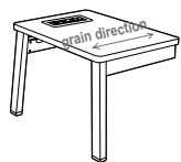
On surface power module on narrow tables
